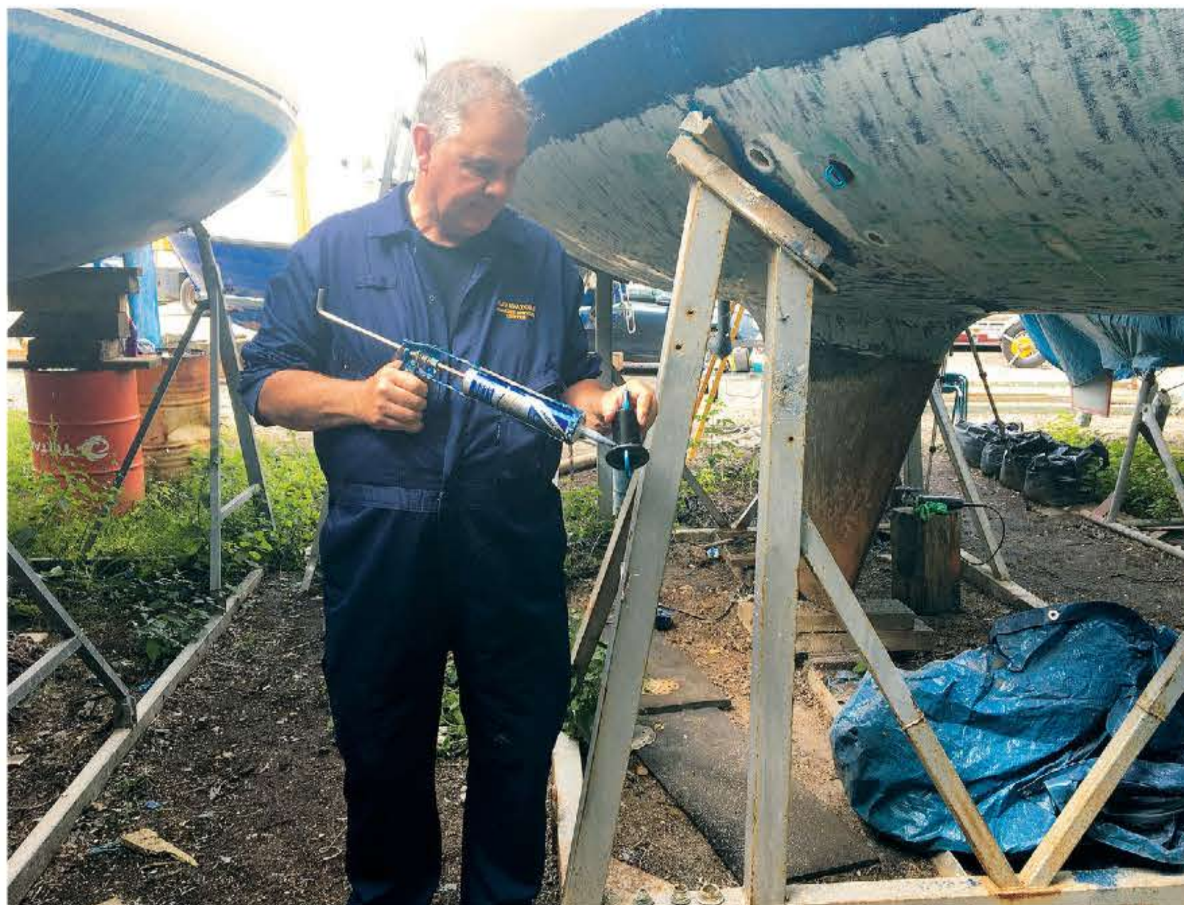
ABOVE Peter Draper adds sealant to the TruDesign skin fitting. Note the application tool is inside it. On the hull you can see he's done one already. TOP RIGHT Cutting out the old fittings. ABOVE RIGHT The old seacocks on Maximus were cut away
